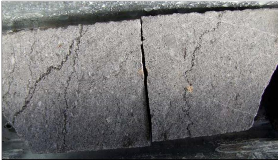
Figure 7.5 – Typical S1 Unit: Fine-Grained Calcirudite with Stylolites
