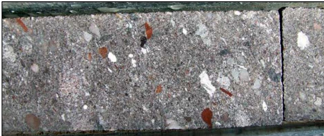
Figure 7.6 – Typical S2 Unit: Conglomeratic Sandstone with Characteristic Red Fragmental Clasts
