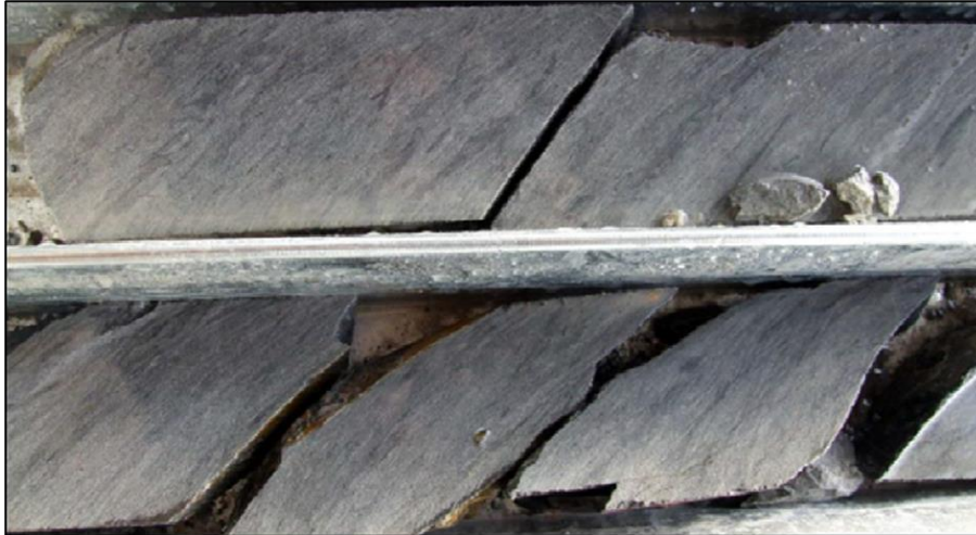
Figure 7.7 – Example of Marl Unit: Grey Marlstone with Deformed Laminations, Drill-Hole BHDD044, 59.2 m
