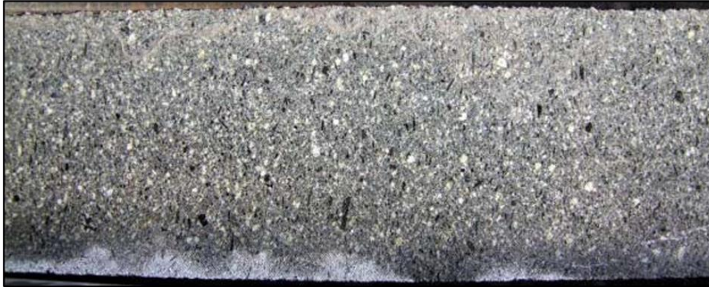
Figure 7.8 – Example of Andesite Intrusive Unit Sill with Phenocrysts of Hornblende and Plagioclase, Drill-Hole BHD010, 101 m
