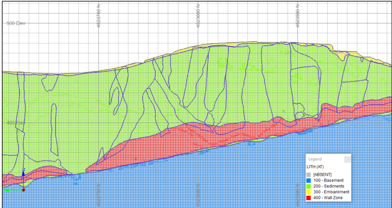
Figure 14-11: North-south section through the Ada Tepe deposit displaying the main lithology units, and mineralised Upper Zone broad mineralisation domains (purple) within the variably mineralised overlying sedimentary rocks of the Shavar Formation (green)
