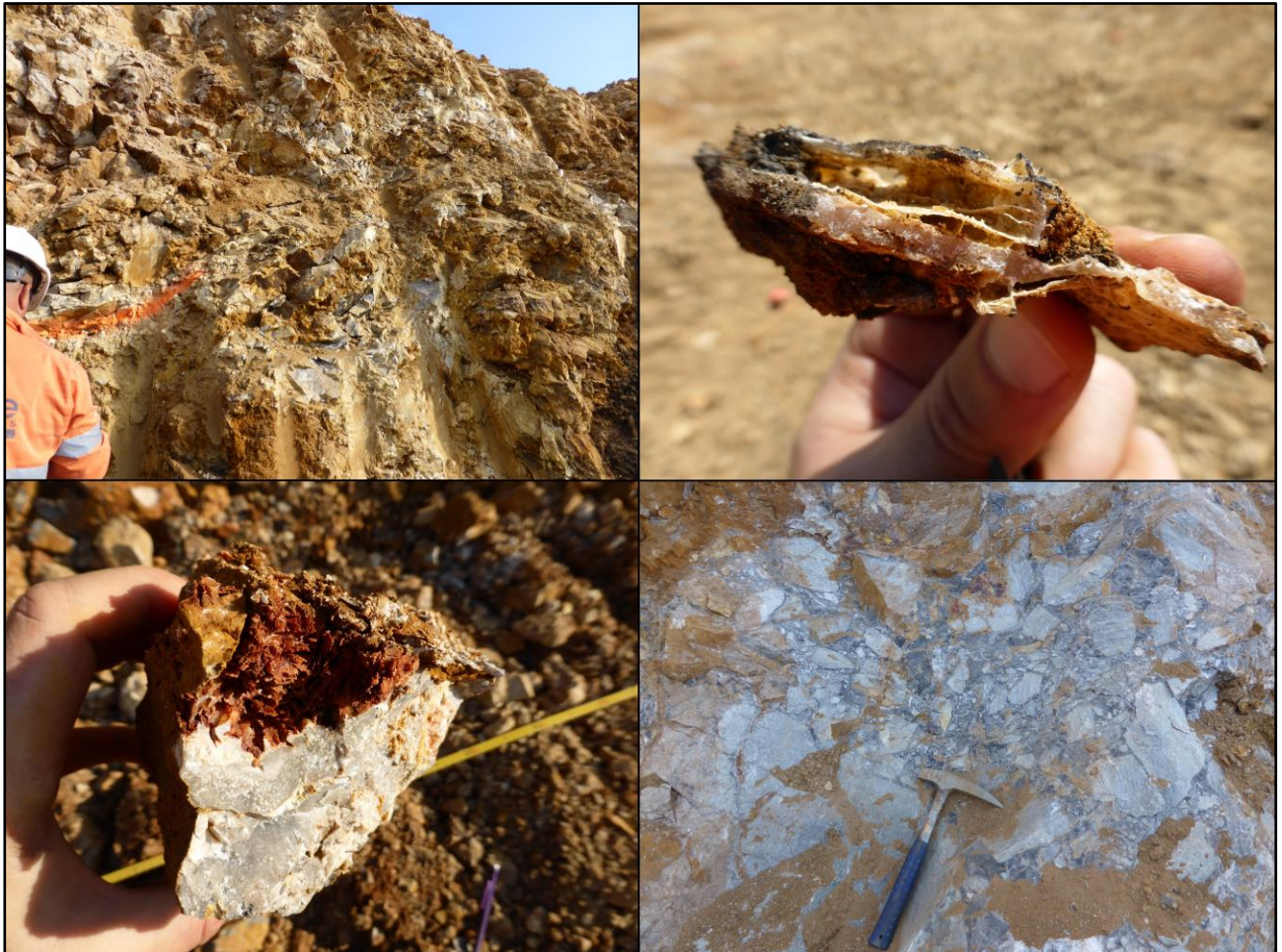
Figure 8-1: Top left – quartz veining through Upper mineralised breccia zone; Top right – silica replacement textures; Bottom left – boiling textures next to silica flooding; Bottom right – brecciation texture in fresh rock exposure near to mineralised zone
