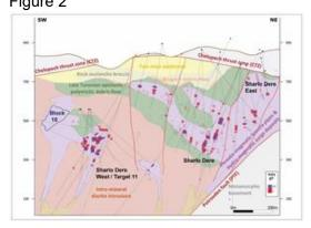
Long-section (A-A') through Sharlo Dere looking northwest, displaying drilling intercepts, interpreted geology, and exploration targets.
