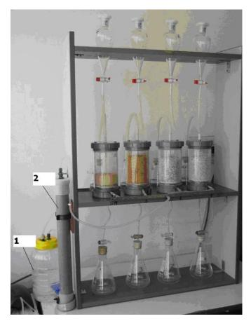
**Fig.4.1.1** – Photo of the kinetic test installation, based on the Humidity Cell Test; 1 – Air humidifier; 2 – Air drying column
