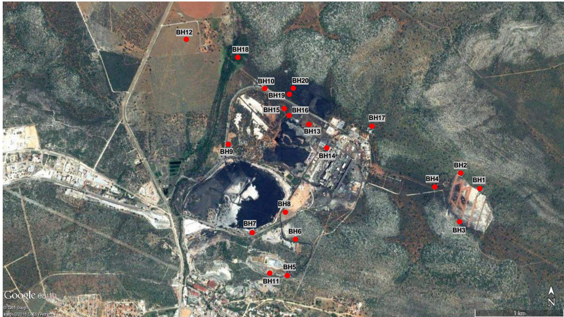
FIGURE 6-2: GROUNDWATER MONITORING BOREHOLE SITES
